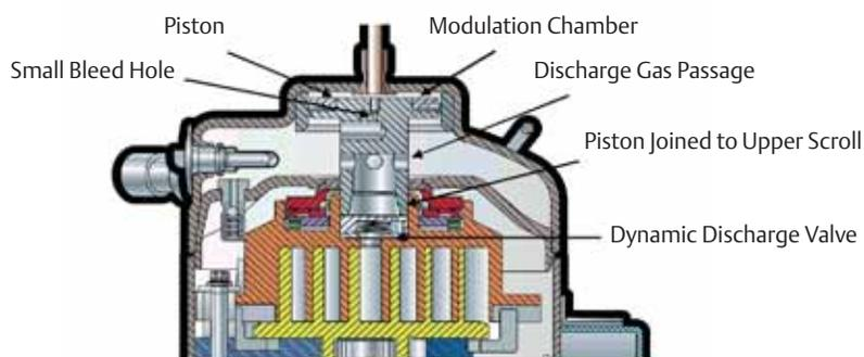
A simple piston in the top cap which is an integral part of the upper scroll is operated by a solenoid valve mounted between the modulation chamber and the compressor suction port.
