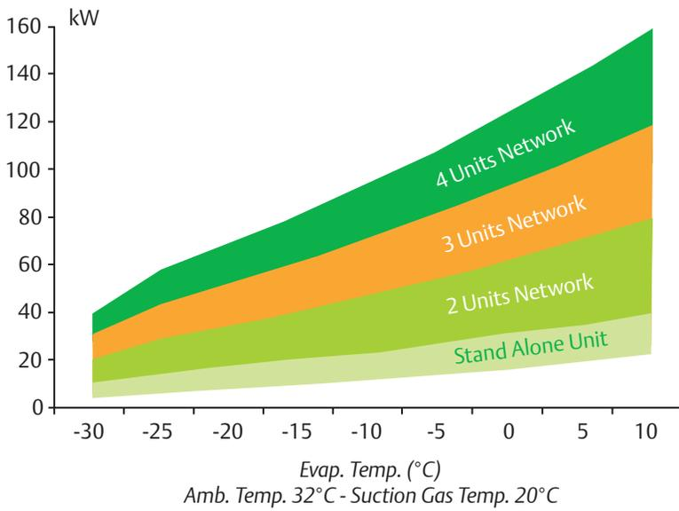
**Outdoor condensing unit for low temperature / capacity per configuration**
