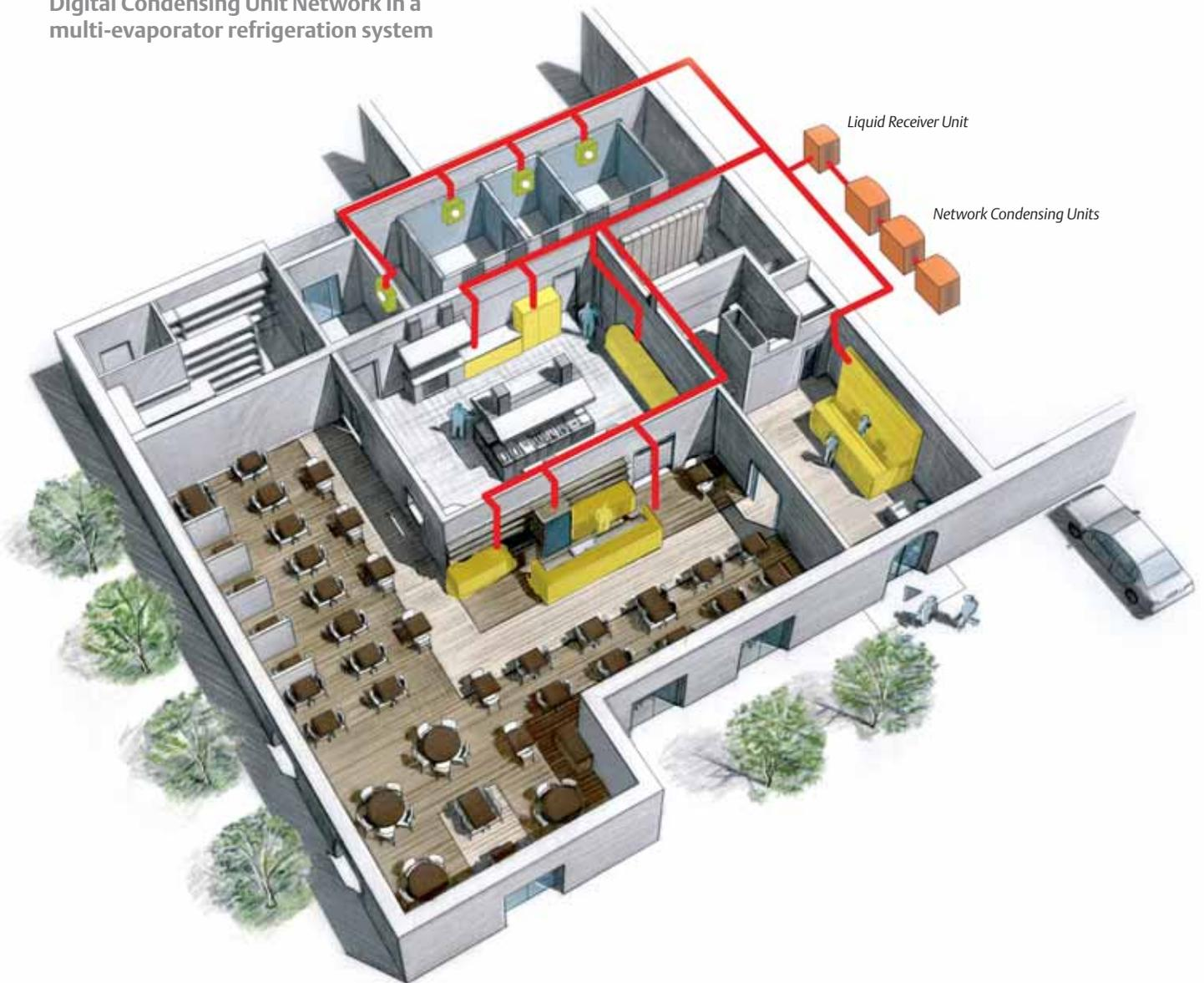
This new concept is defined as “Digital Network” for applications with installed refrigeration capacities up to 90 kW for medium temperature and up to 56 kW for low temperature applications. Aiming for simplicity and speed above all, Emerson Climate Technologies has used technical innovation to reduce not only installation but also operating costs, resulting in complete mastery of energy consumption.
