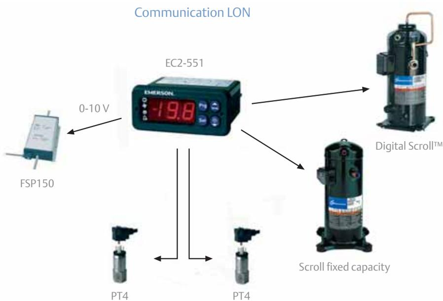
In order to keep electricity consumption to a minimum, Copeland EazyCool™ units use "floating" condensing pressure regulation. An electronic variable speed drive from Alco Controls, FSP150, connected to a pressure transmitter, monitors and adjusts the fan speed to keep it at the minimum required for each unit. Energy saving is the result of maintaining a precise condensing pressure, at the minimum value set via the EC2-551 controller.
